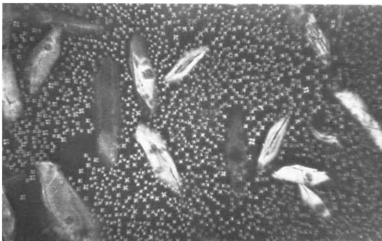
FIGURE 5 Parallelogram texture after rotation of the rods
