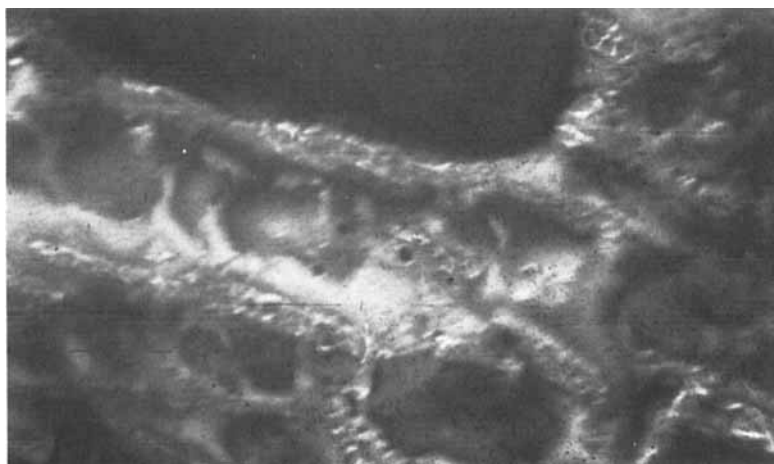
FIGURE 2 N-I two-phase region in the heating cycle
